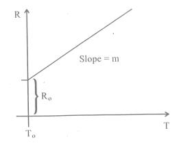
The temperature co - efficient  $(\alpha)$  of the conductor is
