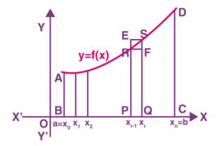
The integral of f(x) is the area of the region bounded by the curve y = f(x). This area is represented by the region ABCD as shown in the above figure. This entire region lying between [a, b] is divided into n equal subintervals given by  $[x_0, x_1], [x_1, x_2], \dots, [x_{r-1}, x_r], [x_{n-1}, x_n]$ .
