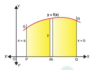
The area under the curve can be assumed to be made up of many vertical, extremely thin strips. Let us take a random strip of height y and width dx as shown in the figure given above whose area is given by dA.
